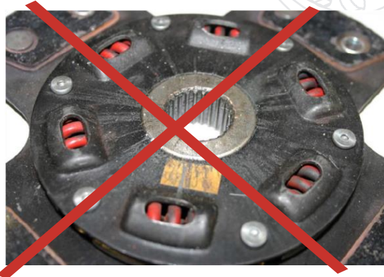
Example of TOO MUCH GREASE.
