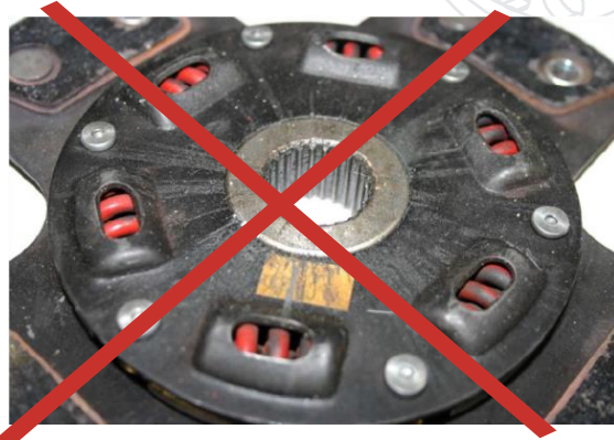
Example of TOO MUCH GREASE.
