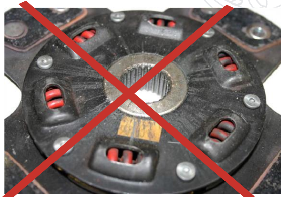
Example of TOO MUCH GREASE.
